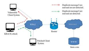
Fig -1: Architecture Diagram for Solution for KRACK Attack
