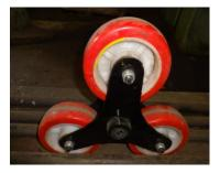
Fig.4.1.1: Assembly of tri-star wheel
