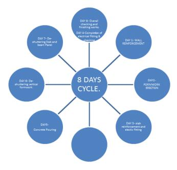
Fig -11: Kumkang formwork work cycle.
