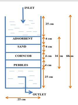
Fig 2(a): Line Diagram of Filter
