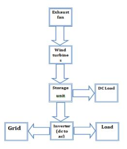
Fig 3.1: Block Diagram of proposed system
