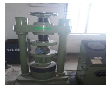
**Fig -6**: split tensile strength test set-up
