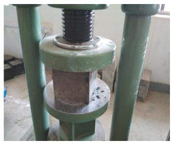
Fig -4: Compressive strength test set-up
