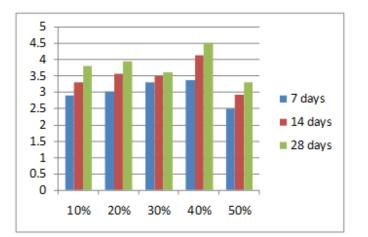
**Fig -6**: Split tensile strength comparison of GGBS, SS and JY Added concrete.
