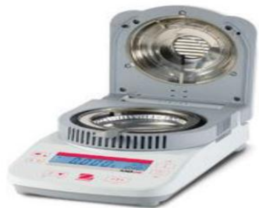
Fig - 4: Moisture analyzer used for measuring the moisture content of the product.
