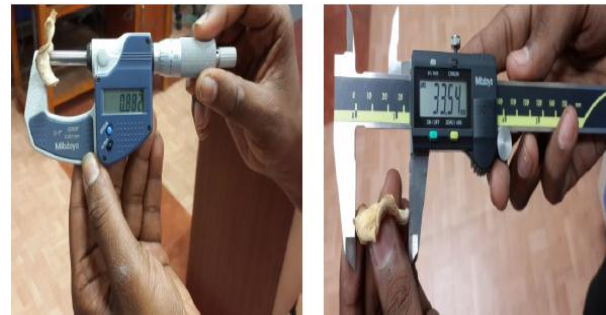
Fig - 3: Instruments used for measuring the product properties (a) Digital vernier caliper (b) Digital micrometer.
