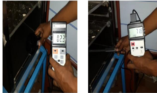
Fig - 2: Instruments used for measuring air properties (a) Anemometer (b) Temperature and Humidity meter.
