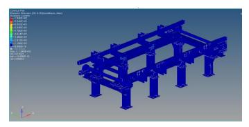
Fig-5: Stress in the conveyor system
