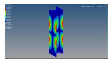
Fig-9: Buckling load in the column
