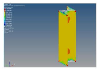
Fig-10: Stresses in the column
