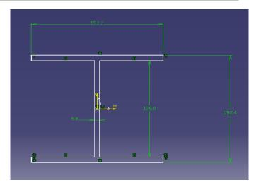
Fig-2: Dimensions of I cross section
