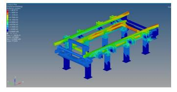
Fig-6: Deflection in the conveyor system
