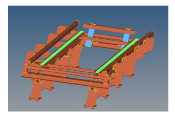
Fig -1: Loading and Boundary Conditions on the Conveyor
