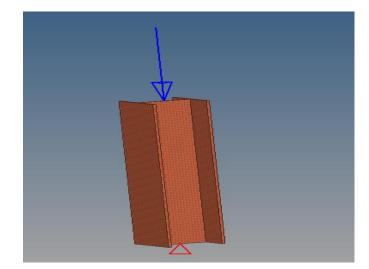
Fig-4: Loading and Boundary conditions on Column
