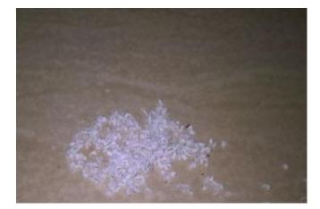
Fig .2. DISCONTINUOUS BRITTLE CHIPS
