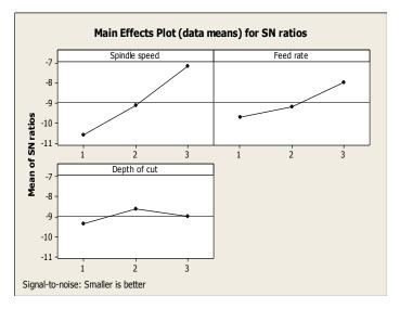
Fig .7.S/N ratio of turning parameters
