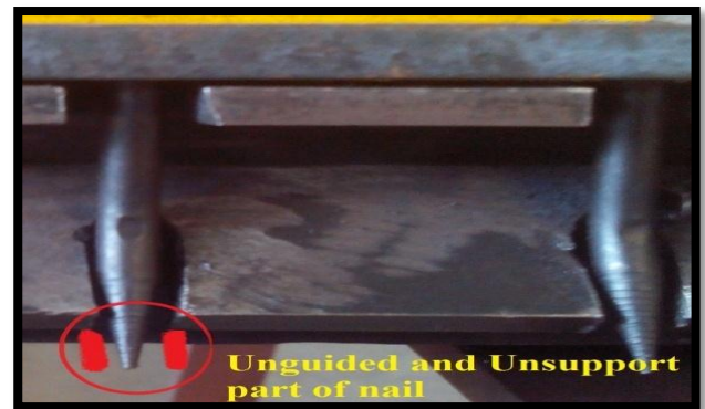
Fig 4.4: - Drawback Existing Jig
