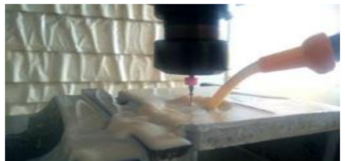
Fig -6: Micro-Drilling using CNC milling machine
