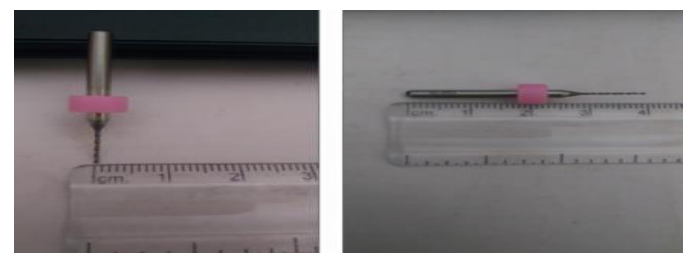
Fig -5: Tungsten Carbide twist drill bit (800μm)
