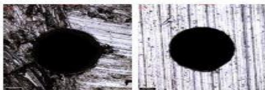
Feed rate: 6mm/min Spindle speed: 4000 RPM (b)
