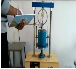
Fig -4: Making of Mould and taking reading from CBR reading
