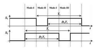
Fig -4: Switching signals for the input boost stage for the proposed converter
