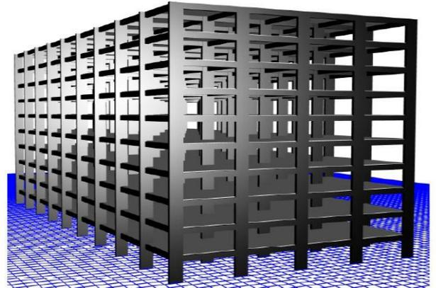
Fig-4. Rectangular building with rectangular columns without dampers
