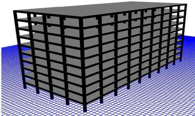
Fig-2. Model of rectangular building with square columns without dampers
