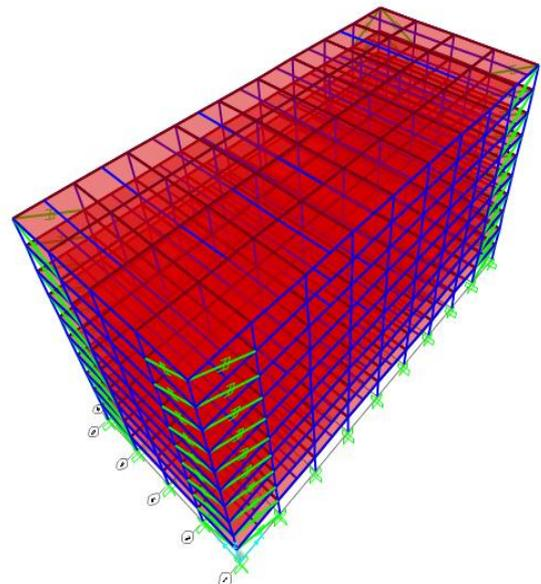
Fig-6. Model of rectangular building with square columns with dampers
