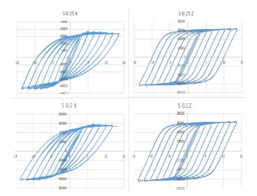
Fig 1. Hysteresis loops of deficient specimens
