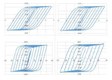
Fig 2. Hysteresis loops of GFRP wrapped specimens
