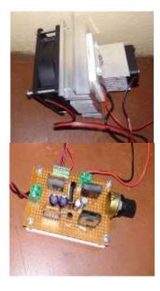
Fig -3&4: Two Peltier Cooling Kit and PWM Controller.
