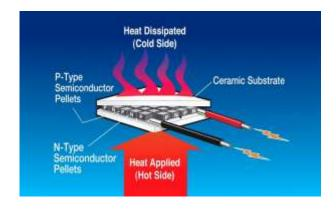
Fig -1: Schematic of Thermo Electric Module Operation – Cooling Mode [7]
