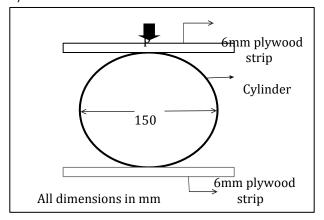
Split tensile test on cylinder specimen
