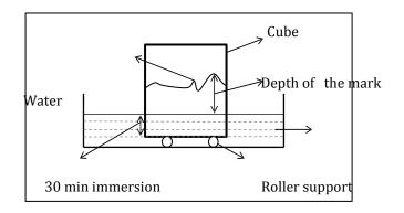
Sorptivity test on cube specimen
