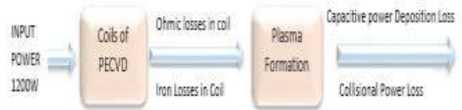
Fig- 2 Flow of losses in PECVD
