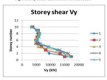
Fig 7. Storey shear distribution in y direction
