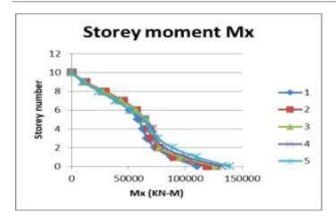
Fig 8. Storey moment distribution in x direction
