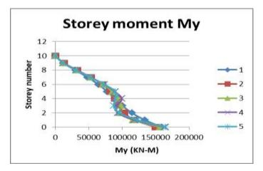
Fig 9. Storey moment distribution in y direction
