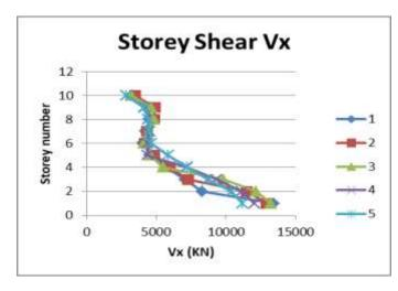
Fig 6. Storey shear distribution in x direction
