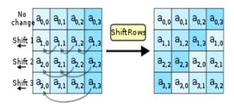
Figure 3: In this figure each byte is shifted cyclically.
