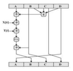
Figure 7 . Process of 512 bit message block
