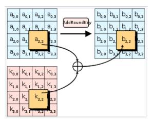
**Figure 4.4**: Each byte of the state is combined with the byte of the round sub key using XOR operation.
