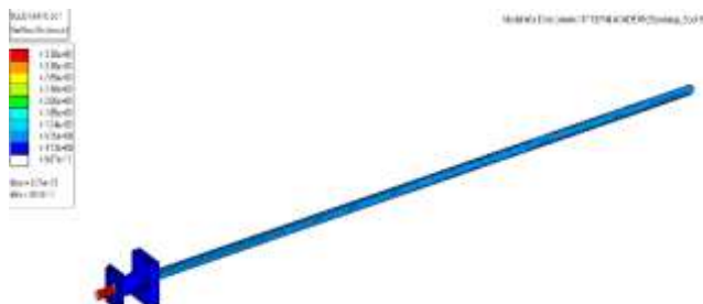
Fig 4.2: Maximum Stress 119 MPa in Lance tube
