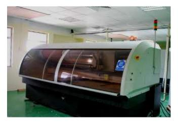
**Fig No. 2** : Lenz PCB drilling machine
