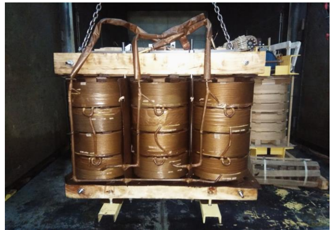
Fig -2: Transformer with wooden clamping
