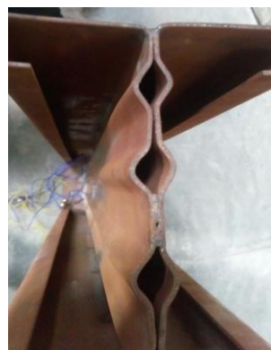
Fig -7: Failure pattern of column
