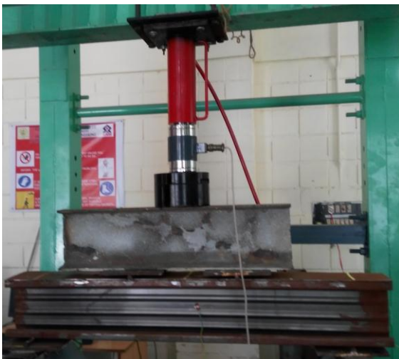
Fig -4: Experimental test setup for flexure test
