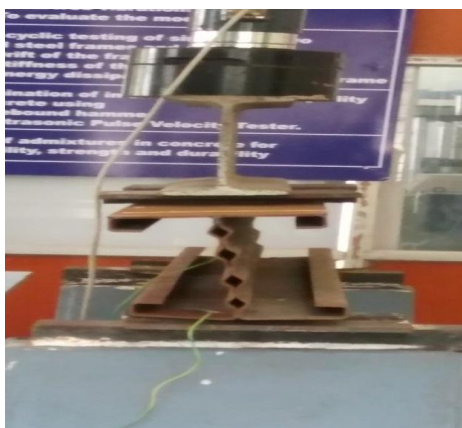
Fig -5: Failure pattern of beam
