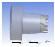
Fig-4: Three dimensional view of M Lobe chevron nozzle model
