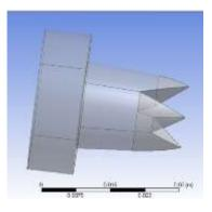
Fig-3: Three dimensional view of asymmetric chevron nozzle model.
