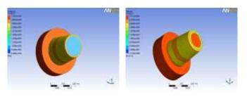
Fig-7 pressure distribution of baseline nozzle model Fig-8 velocity distribution of baseline nozzle model
