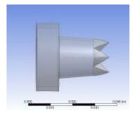
Fig-2: Three dimensional view of chevron nozzle model
