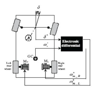
Figure 5: Electronic controlled differential [5]
