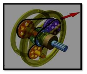
Figure 6: Belt driven differential [11]
