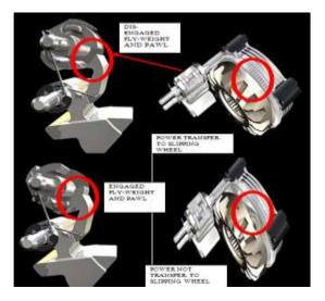
Figure 9: Locking differential by centrifugal force [12]
