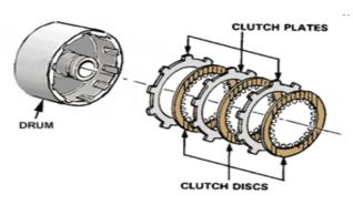
Figure 3: Locking differential by clutch pack [8]
