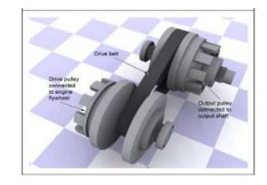
Figure 7: Continuous variable transmission differential [1]
