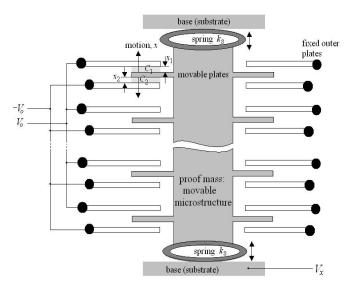
**Fig -4**: Accelerometer structure. Proof mass is attached through springs (kS: spring constant) at substrate.
