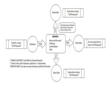
Fig -5: MQTT Broker based architecture
