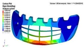
Figure-19: Displacement for Mode 1 Modal Analysis
