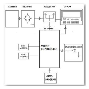
Fig -1: Block Diagram of Enhanced Railway Track Security System
