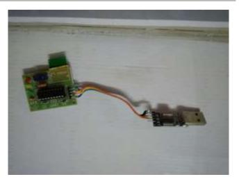
Figure 2. RF Transceiver
