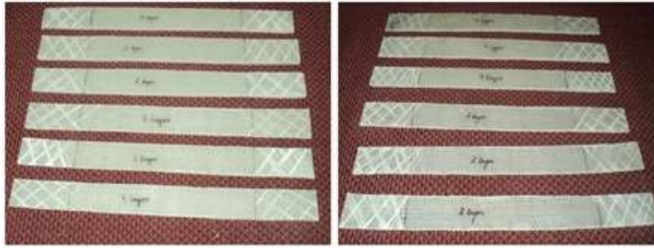
Fig.-7: Samples for tensile testing
