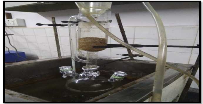
Fig 3.2.5: Extraction of Oil using Soxhlet Apparatus.
