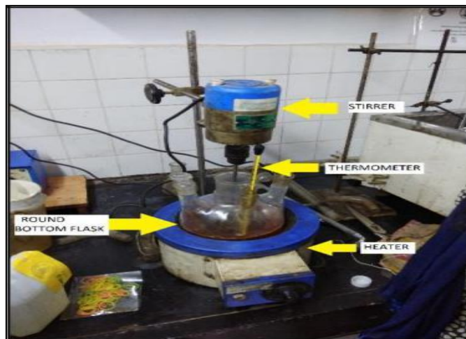
Fig 3.1.2: Round Bottom Flask Apparatus
