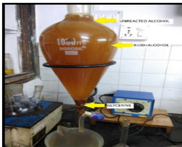
Fig 3.2.5: Before & after image of Biodiesel in settling apparatus
