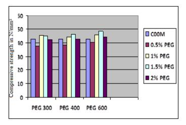
Fig 4. Effect of self-curing agents on 7<sup>th</sup> day Compressive Strength of concrete
