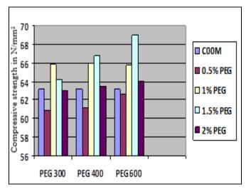
Fig 5. Effect of self-curing agents on 28<sup>th</sup> day Compressive Strength of concrete
