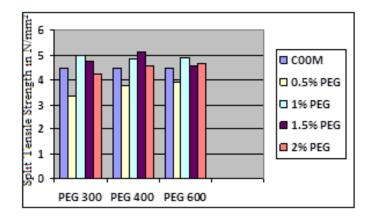
Fig 6. Effect of self-curing agents on 7th day Split Tensile strength of concrete
