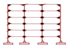
Fig-2: Bare frame system
