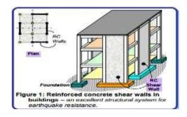
Fig-3: Location of Shear walls in RC buildings
