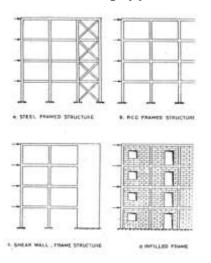
Fig-1: Lateral load resisting structures
