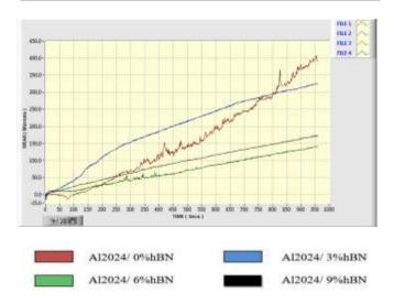
**Fig-6:** Variation of wear v/ s time with the addition of hBN Reinforcement under 20N load and 0.5m/s velocity.
