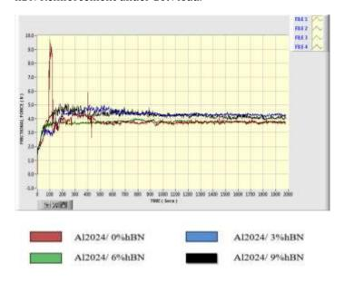
**Fig -4**: Variation of friction force v/ s time with the addition of hBN Reinforcement under 10N.
