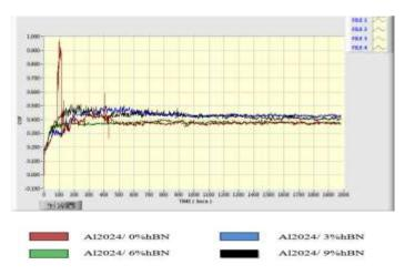
**Fig -5**: Variation of COF v/ s time with the addition of hBN Reinforcement under 10N load.
