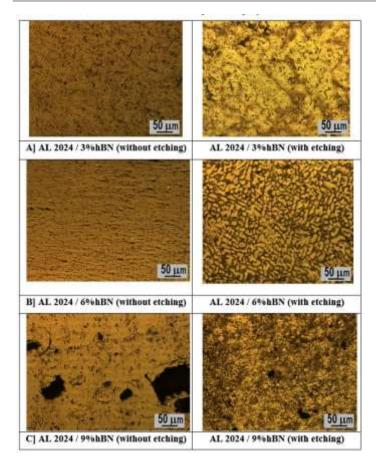
Fig -2: Optical micrographs of MMCs
