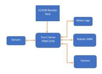
Fig -1: Block Diagram (Receiver Block)
