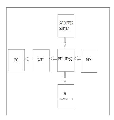
The transmitter section consists of PIC18F452, Power supply, GPS, RF Transmitter, WiFi. When the RF Transmitter is in the
