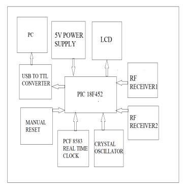
A receiver section is especially focused on PIC18F452, RFID Tags, Real Time Clock( PCF8583), Power supply. The presence of RFID Tag is monitored by RF receiver. The received information of student is then stored in the record with the time and date. The time and date are saved with the help of a real-time clock.
