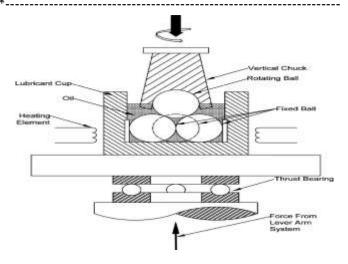
Fig. 1 Schematic diagram of four ball tester
