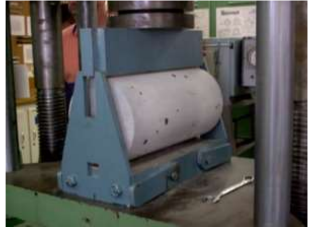
Fig. No-2: Split tensile test
