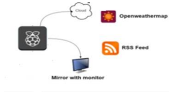
Fig -2: Architecture of a Smart Mirror
