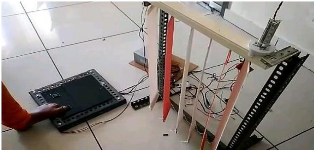
Fig -6: Vertical Blinds Movement Control
