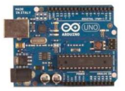
Fig – 1: Arduino UNO Board
