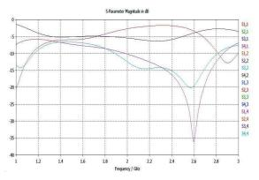
Fig. 5. S-parameter results of the simulation in HFSS microwave software of the directional coupler cut at 45° angle at edges
