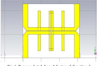
Fig. 6. Proposed stub-based design of directional couplers.[5]
