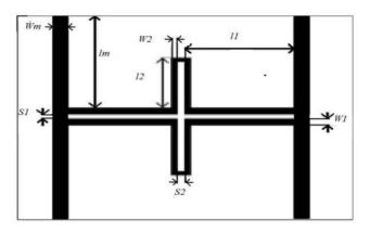
Fig. 1: Top view of the design layout of the earlier proposed high directivity and tight coupling coupler. [4]
