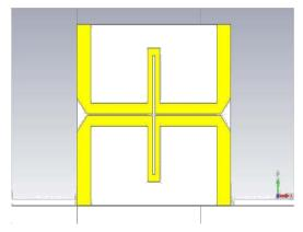
Fig. 4. Coupler edges cut at 45° angle.
