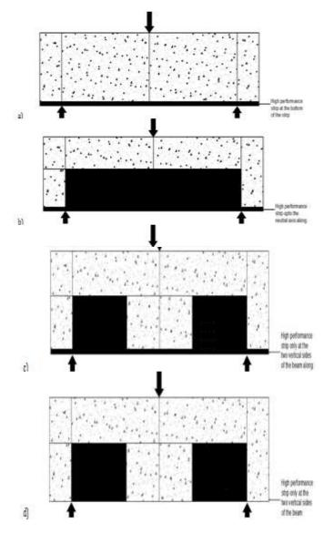
Fig: 12. a) Strip placed on the soffit of the beam
