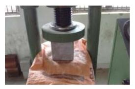
Fig 5: Testing of Cube in CTM
