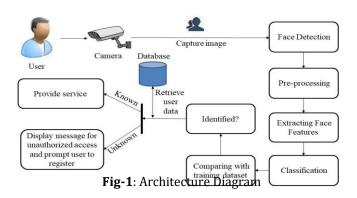
The proposed system consists of a camera that captures images of a user. These captured images are then sent to the Face Recognition System(FRS) which further does preprocessing, face detection and feature extraction. Classification step is used to identify whether the user is authorized or not. If it is an authorized user, service is provided to it in the form of virtual assistant. Otherwise, the user is prompted to register with the admin.
