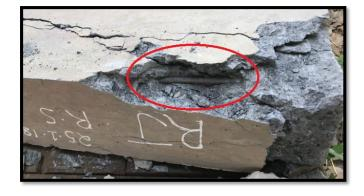
Fig -4: Cover failure and reinforcement exposure of rebar specimens
