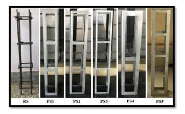
Fig -1: Rebar and PCS reinforcements used for the study
