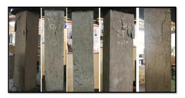
Fig -2: Crack pattern PCS square specimens
