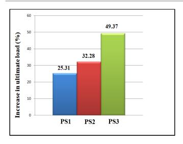
Chart -2: Bar chart showing the effect of steel sheet thickness
