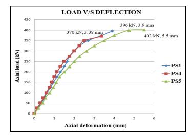
**Chart -3:** Load v/s deflection curve showing the effect of transverse steel width and spacing
