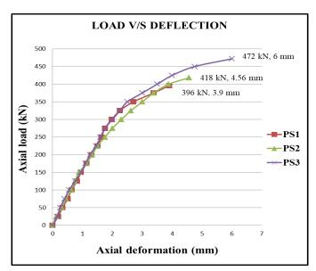
**Chart -1:** Load v/s deflection curve showing the effect of steel sheet thickness
