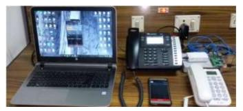
Fig -12: Hardware set up of Proposed IP-PBX system
