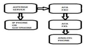
Fig -6: Block Diagram of Proposed IP-PBX system
