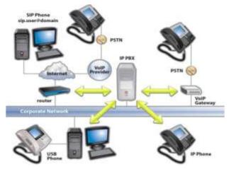
Fig -5: Basic VoIP network Layout
