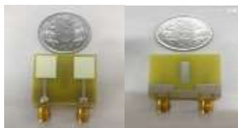
Fig-3 photograph of fabricated antenna
