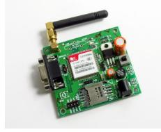
Figure 1: GSM module
