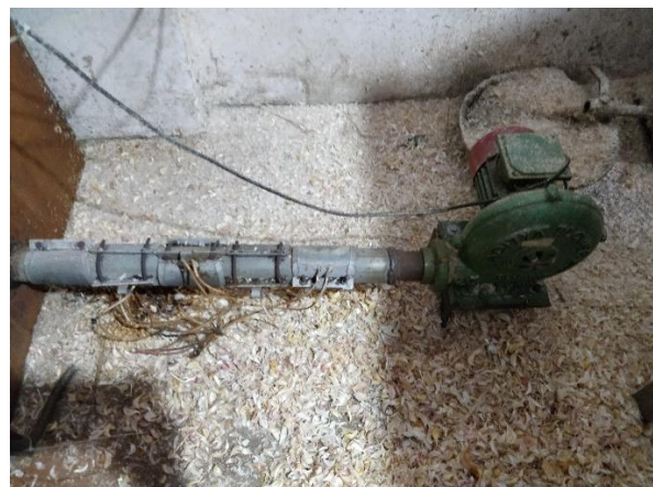
Fig- 1.4: pipe and blower arrangement
