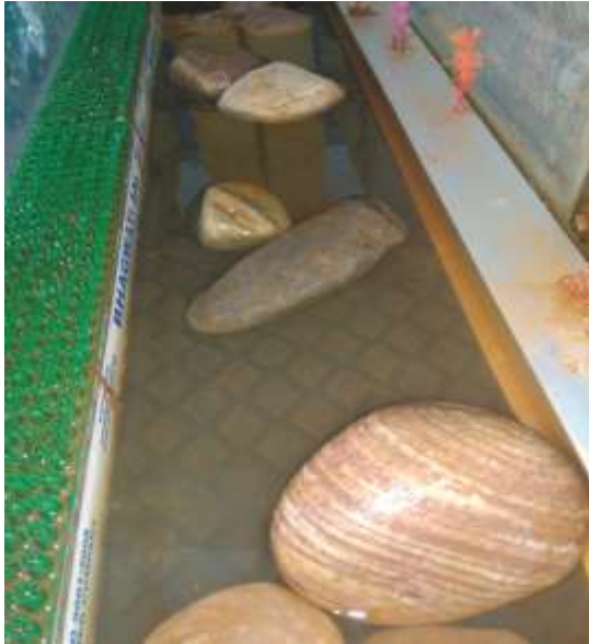
Fig -2: Cross section of the compound channel with the bed resistance PVC along with the Boulders.
